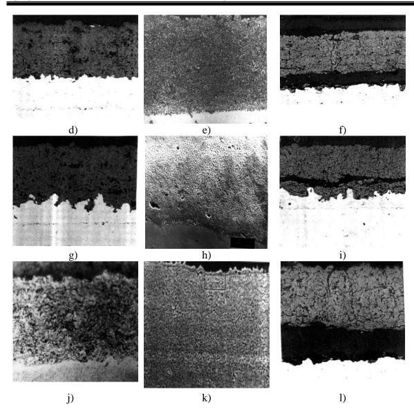
**Figure 1.** Microstructure of heat-shield coatings of the NiCrAlY-ZrO<sub>2</sub>-7%  $Y_2O_3$ . 400. a), b), c) - APS; d), e), f) - SAPS; g), h), i) - VPS; j), k), l) - HVOF; a), d), g), j) - coating after deposition; b), e), h), k)- coatings after thermal treatment (1100 °C, 2 hours - vacuum); c), f), i), l) - coatings after thermal cycling (heating up to 1170 K, holding for 15 minutes, cooling down to room temperature with compressed air).
